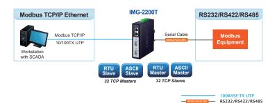
The advantage of having the IMG-2X00T Series is to assist users to build an industrial environment between the Modbus TCP/IP Protocol and the Modbus RTU/ASCII Protocol easily, thus offering an application solution to the industrial control equipment without Ethernet ports and the industrial control equipment can only control through an industrial PC workstation or industrial control panel.
