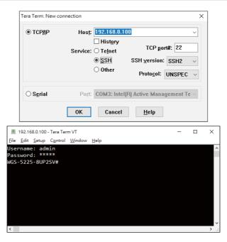
Figure 6-1: Wall-mount Managed Switch SSHv2 Login Screen
