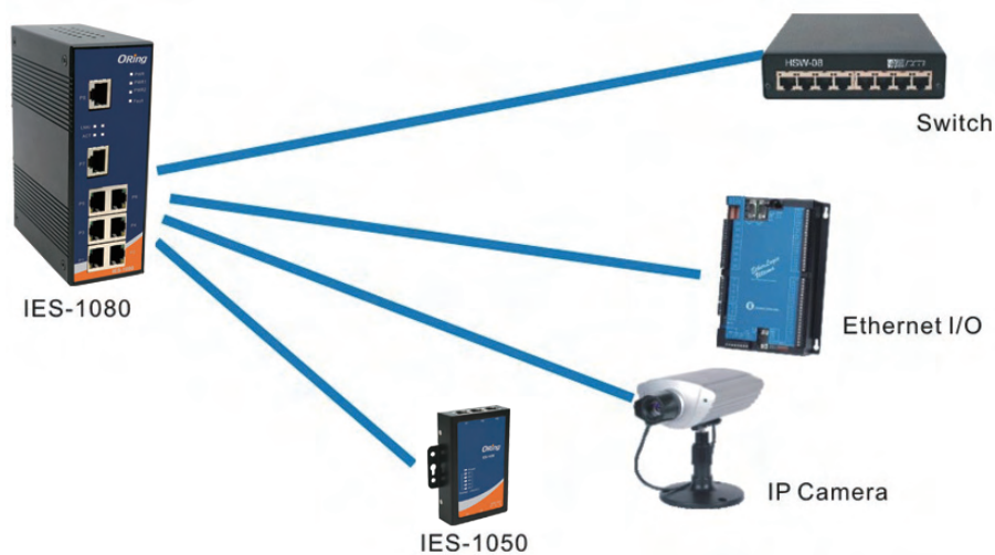
Connections of Ethernet devices
