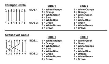
Figure B-1: Straight-through and Crossover Cables
