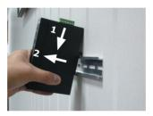
**Step 5:** Lightly pull out the bottom of the DIN rail from the track to remove.
