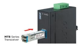
Figure 3-1: Plug in the SFP+ Transceiver
